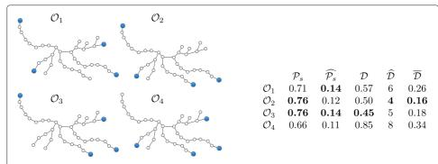
**Fig. 4** A tree with different sets of k=4 observers (*blue*). The table displays the values of different metrics for the observer sets. The best values for each metric are in *bold type*. The remaining possible choices of k=4 observers within the leaves set are omitted either because they are equivalent to one of the placements considered or because they do not optimize any of the metrics examined
